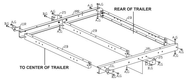
Figure C: Rear Bed Rail Assembly
